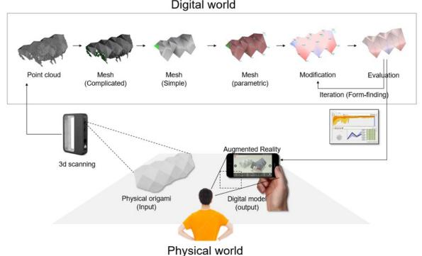
Figure 1: A dataflow diagram between physical and digital model
