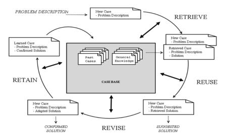
Figure 3: The 4R's cycle for CBR system development
