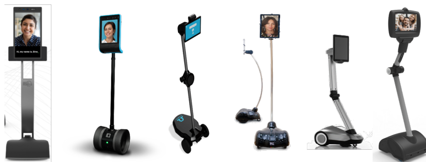
Figure 5. Telepresence Robot Models, from left to right: GoBe [10], Double 3 [11], Ohmni Robot [12], BotEyesPad++(Samsung Galaxy S7)[13], PadBot P2 [14], UBBO Expert [15]
