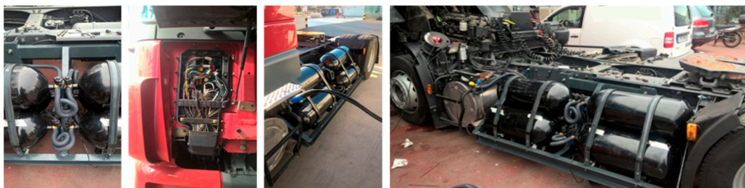
Figure 6. Indicatives screenshots from the retrofitting equipment used for the dual-fuel system.
