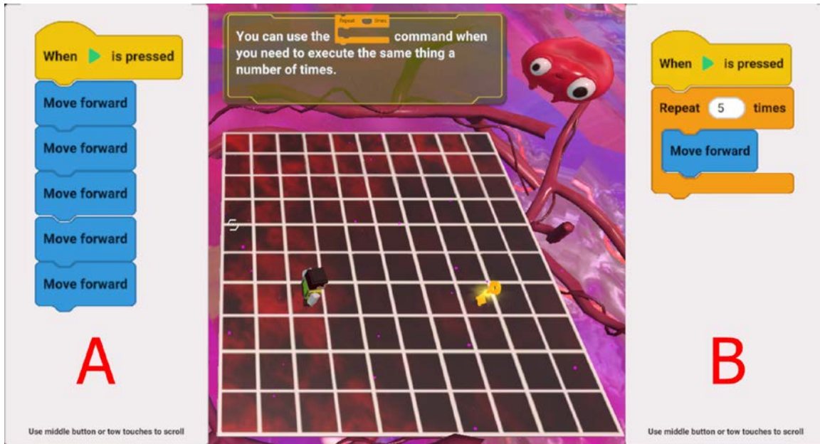
Figure 4. An example of two solutions to a puzzle: (A) uses the sequence structure, (B) uses the iteration which is more efficient programmatically.
